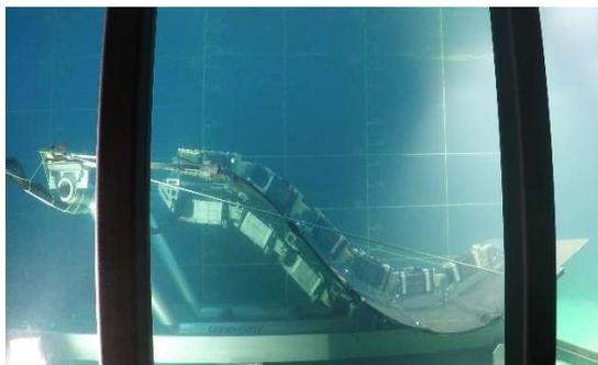
EEL tidal prototype (10KW output)
